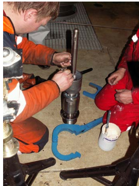
Figure 6: The Temperature Probe assembled in its housing is attached to the inner core barrel head assembly.
