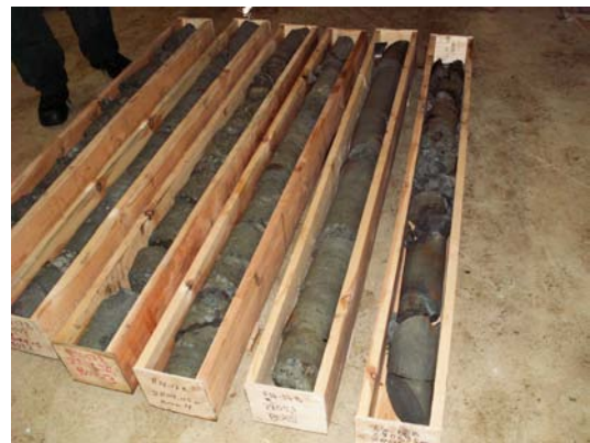
Figure 12: Core removed from Core Barrel and boxed for examination.
